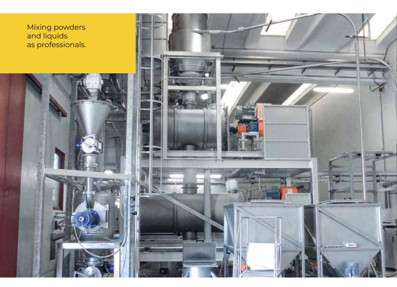
From the receiving of the material in any format, from bulk to bags, the mix recipe is automatically composed by sieving and conveying each ingredients from its source, and dosing precisely the quantity needed.
