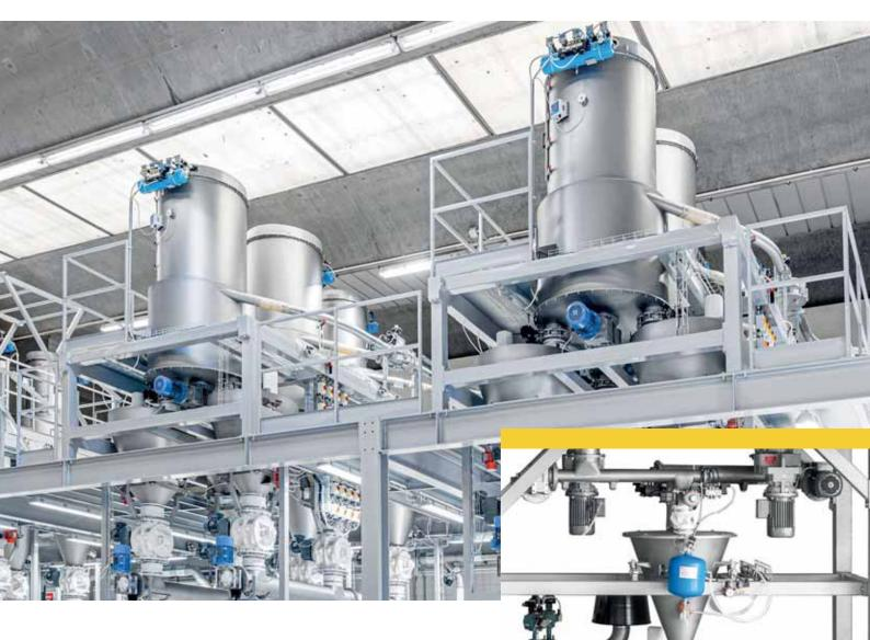
Ingredients are dosed in the desired quantity directly from the storage containers, guaranteeing complete traceability.
